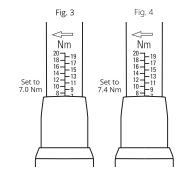
To operate, gently apply pressure to the torque while 'gripping the knurled handle, being careful to listen for the "Click" when the desired torque is reached. Do NOT over tighten past this point.
