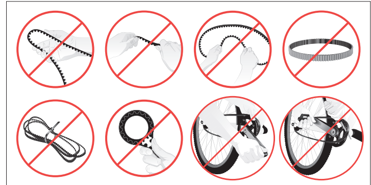
Fig. Types of damage
